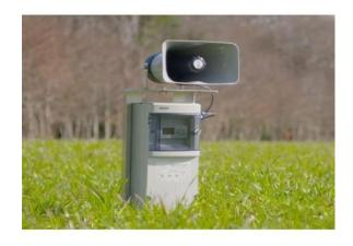
Fig.5 Ultrasonic Electronic bird repellent
